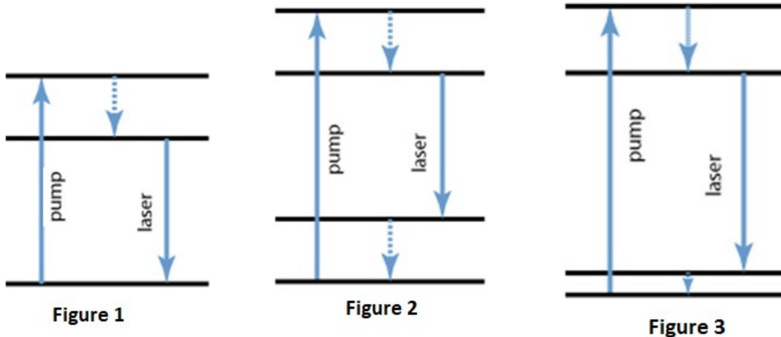
Fig 1: a three-level system, the laser transitions ends on the ground state. Fig.2: a four-level system, the laser transition ends on a level above the ground state, which is quickly depopulated e.g. via phonons. Fig 3: a quasi-three-level system, where the lower laser level has some population in thermal equilibrium.
